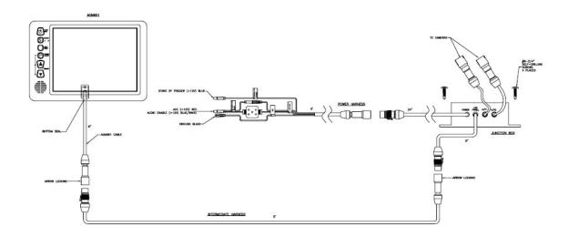
Install the **AOM713WP** monitor panel, Intermediate harness, junction box and wiring harness in place of the old system. Your camera cable will connect into the **TO CAMERA** inputs.
